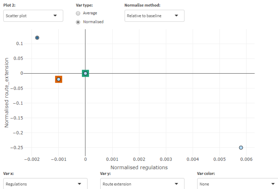
Figure 6 - Another possible way to answer questions number 4, 5, and 6: the solutions are presented scaled with respect to the baseline (as in the PCP in Figure 4). The point in orange is improving the two indicators in both dimensions and therefore it is drawn at South-West w.r.t. to baseline (in green).
